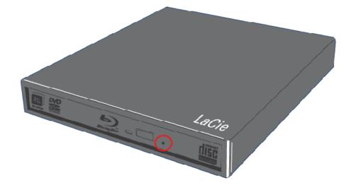
3. Insert a small metal poker, such as the end of a paper clip, into the emergency eject hole until it presses against the manual eject mechanism. You will feel the mechanism eject the disc tray.
