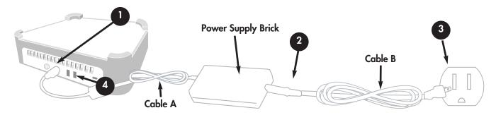
There are two cables that are supplied with the power supply: one cable (A) connects to a power outlet, such as a wall outlet or a surge protector; and the other cable (B) connects to the LaCie drive.
