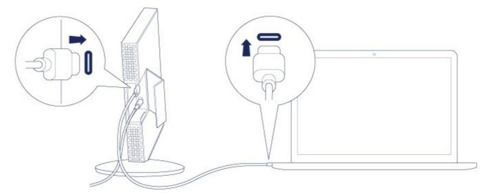
• The image below shows a connection to a computer with a USB 3.0 or 2.0 Type A port.
