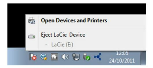
Select **Eject** for the device you want to unmount. A message appears notifying you that it is safe to remove the drive.
