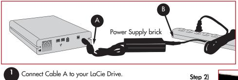
There are two cables that are supplied with the power supply: one cable (A) connects to the LaCie drive; and the other cable (B) connects to a power outlet, such as a wall outlet or a surge protector.
