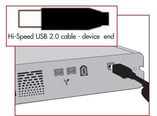
**Tech Note:** To achieve Hi-Speed USB 2.0 data transfer rates you need to be connected to a Hi-Speed USB 2.0 host interface. Otherwise, you will be limited to USB 1.1 speeds. For more information, please see sections: 5.3. Optimizing Data Transfers 5.3.2. Hi-Speed USB 2.0 Ports And Performance.
